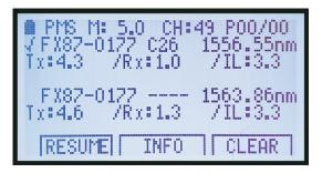
Valid, Passed, Failed and Missed channels are detected and those with an unexpected ID are reported as rogue channels. Technicians can compare the Total channels versus the predefined channel plan to see what has been received.
