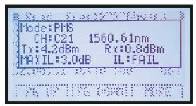
The insertion loss is accurately derived from the ratio of the transmitted optical power reference and the received power. Programmable loss thresholds stored in the FX82s memory are used for pass/fail certification at defined test points/locations.
